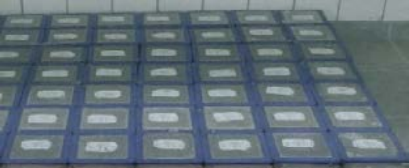
Figure 8: Concrete Sample Moulds
