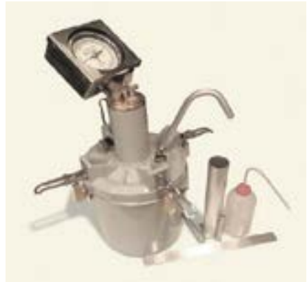
Figure 7: Air Measurement Device
