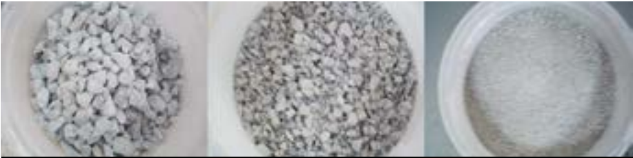
Figure 3 : Aggregate Piles of Different Grain Diameters
