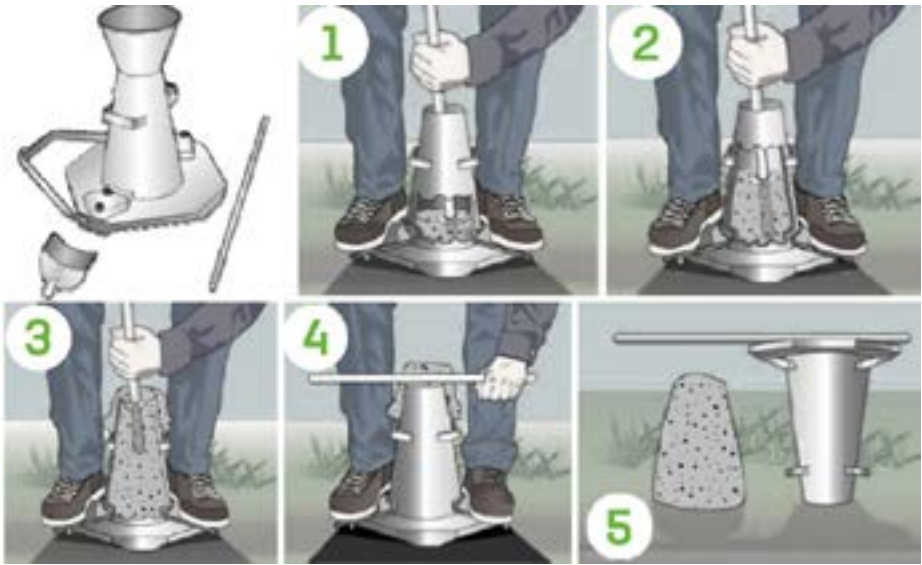
Figure 6: Slump Test
